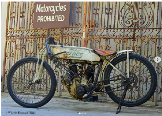
Left- Thor Boardtracker - This 1913 Thor Model SR Boardtrack racer on display at Dale's WTT is the only known twin cylinder example of a Thor racing machine. It features original paint and is run regularly for visitors. The engine is 61 cubic inches and is capable of speeds in excess of 80 mph.
