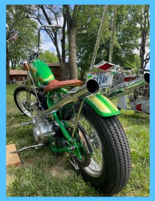
This 1939 Knuckle chop is a very recent build. It features a custom single downtube frame. Jack made the sissy bar, exhaust pipes, top motor mount, front brake rotor and carrier, and the hand and foot controls. He had to modify the dual piston brake caliper to single piston and he modified the early Sportster oil tank to fit the left side chain drive. This bike and the '69 FLH Shovelhead below really show Jack's artistry and his love for the choppers of the 60's and 70's.
