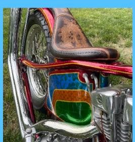
A lot of home made fabrication went into this build. Jack made the frame jig and the frame, the front end jig and the extended springer on his Shovelhead
